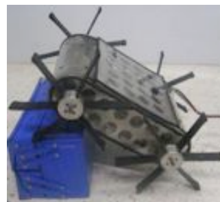
Fig. 1 A Leg-Wheel Hybrid Vehicle with adjustable number of spokes
