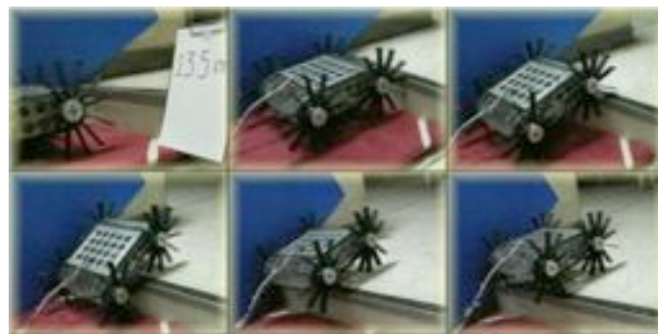
Fig. 11 Twelve-spoke wheel climbing up the stairs
