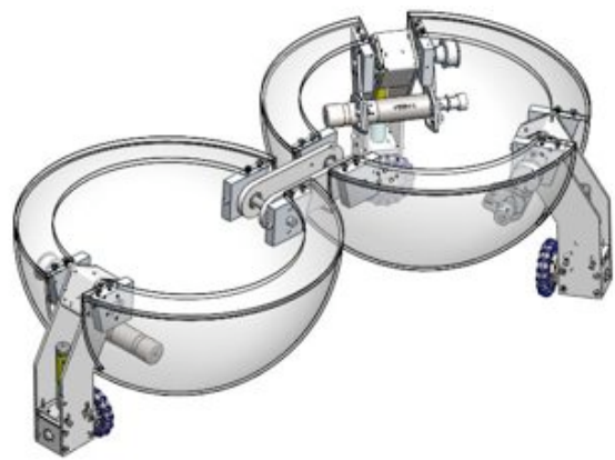
Fig. 3. Reconfigurable Robot after transformation
