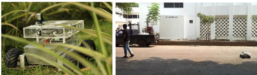
Fig. 1. All-terrain robot for tracking and pursuit of arbitrary target objects using a monocular camera.
