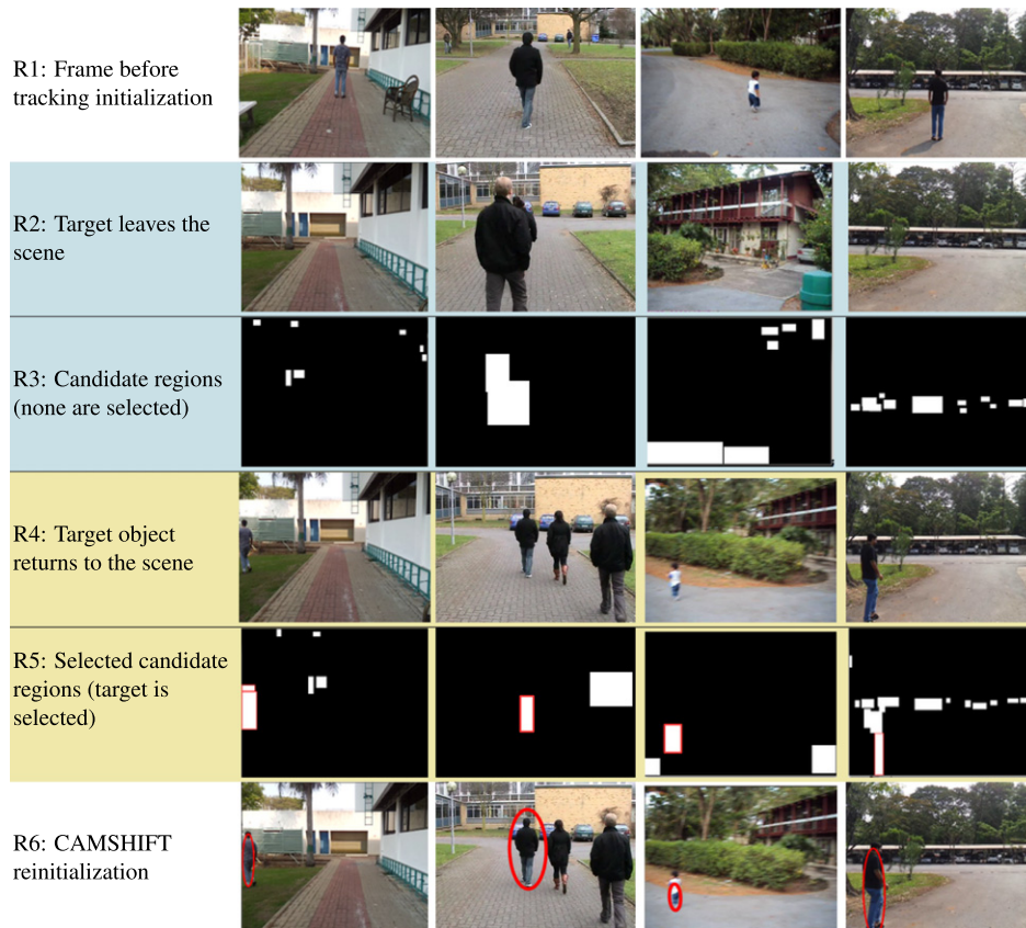
Fig. 9. Experiment IV results. The proposed method was tested in different outdoor environments with different background and target objects. Each column shows images from a different video. Rows show results of each step of processing. Blue colored rows show processing when the target is not in the scene. Yellow colored rows show the same processing steps when the target returns to the scene. (For interpretation of the references to colour in this figure legend, the reader is referred to the web version of this article.)
