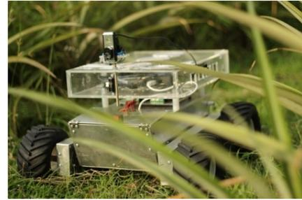
Fig. 1. All-terrain robot for tracking and pursuit of arbitrary objects using a monocular camera.
