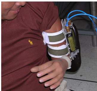
Fig. 9. Prosthetic arm actuated by artificial muscles
